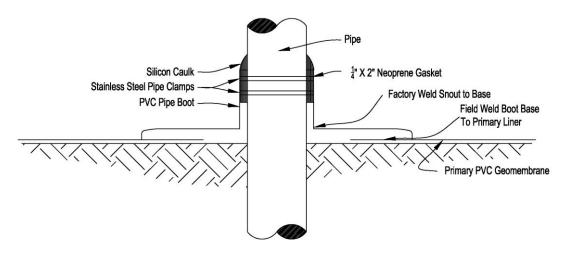
Pipe boot material shall be equal to or greater in thickness than the specified primary liner.
